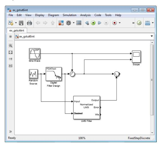
The positive input to the second Sum block is the sum of the input signal and the low frequency noise, s(n) + y. The negative input to the second Sum block is the LMS Filter block's best estimation of the low frequency noise,
