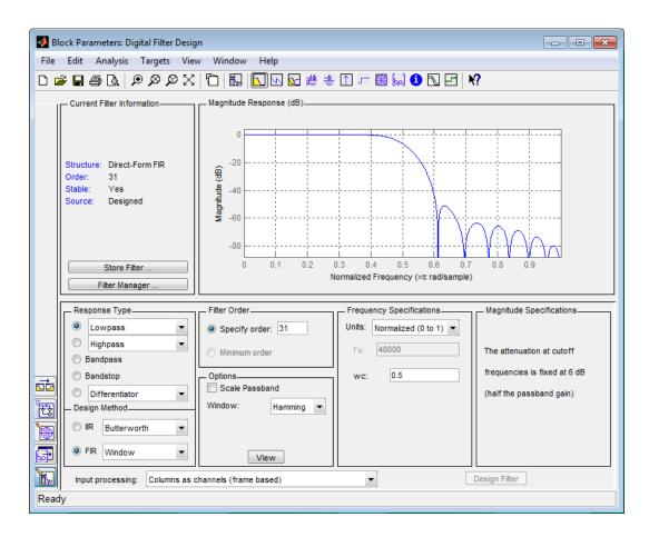
You have now designed a digital lowpass filter using the Digital Filter Design block.
