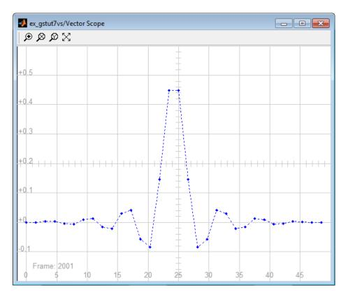
You can simultaneously view the behavior of the system in the Scope window. Over time, you see the error decrease and the approximation of the input signal more closely match the original sinusoidal input signal.
