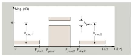
In this example, a sampling frequency of Fs = 48 kHz is used. This bandpass filter has the following specifications, specified here using MATLAB code:
